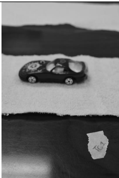
Friction Roll. Use masking tape to mark the distance the car rolls on each track.
