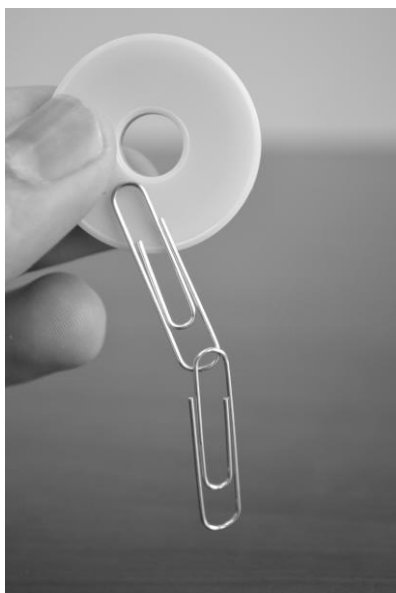
Magnet Chain & Stack. Touch a second paper clip to the paper clip that's on the magnet. The second paper clip is magnetized without directly touching the magnet.
