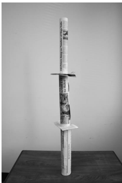
Paper Tower. Sample tower made from newspaper and masking tape.
