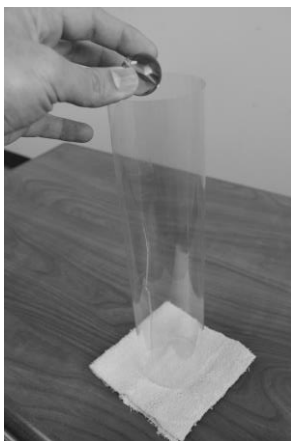
Balls, Bounce & Billiards. The "test chamber" stands upright, with one opening on a folded piece of felt. Drop each ball from the top.
