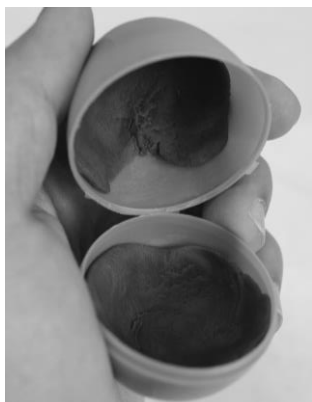
Egg Roll. Example of an engineered egg that can roll down a ramp. The weight of the play dough is evenly distributed inside the egg.
