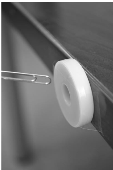
Floating on Air. The paper clip will levitate if held within the magnet's magnetic field. (Scotch tape is pictured instead of masking or painter's tape so that the magnet is visible.)
