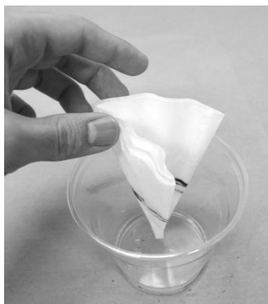
Act. 3, Cool Chromatography. Place the folded coffee filter wedge in the cup, point down. The tip of the wedge will be submerged in the small amount of water in the cup.
